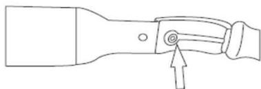
Secure the backstrap into position by tightening the screw and nut.
