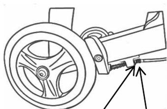
Adjust brake tension, Loosen the locking nut, and turn the adjustment screw clockwise/ counter clockwise
