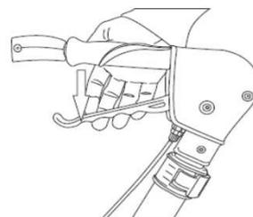
Push down on brake handle to lock the brake into PARK.
