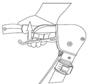
Pull up on brake handle to slow down or to release the parking brake.
